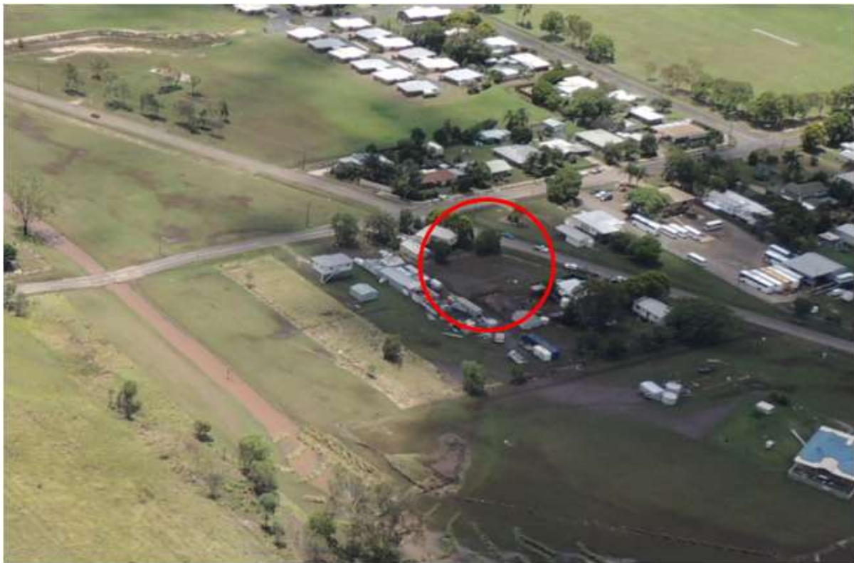
Figure 9 – Post 2013 flood photo – note sediment deposition.
