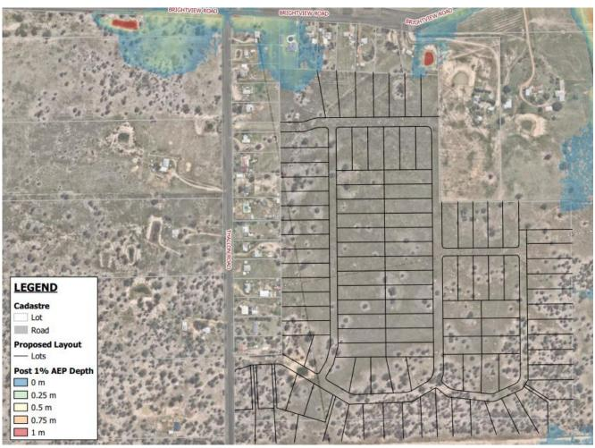
Figure 1: Post Development Flood Results 1% AEP Depth
