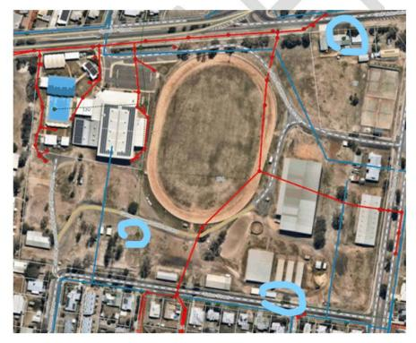
Figure 31: Recommended Sanitary Drainage Connection Points
