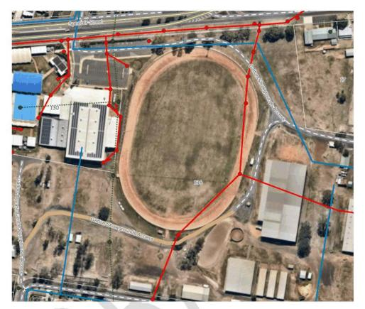
Figure 26: LVRC Stormwater Infrastructure
