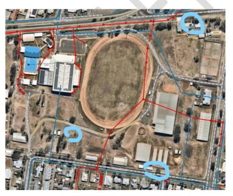
Figure 31: Recommended Sanitary Drainage Connection Points
