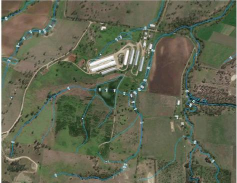
Figure 3: Drainage channels surrounding the poultry farm
