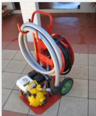
Figure 13. Fire pump may be portable, or fixed in position, so long as it is protected as the fire front passes.
