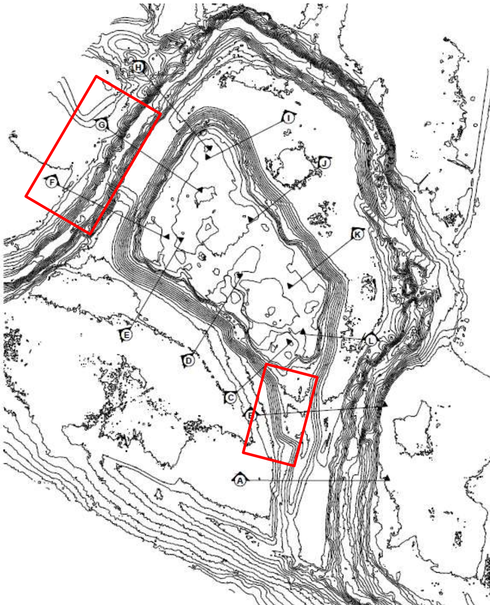
Figure 1 – extract from Golders report – contour plan of rehabilitated quarry with the western spillway and eastern inlet nominated (in the red boxes).
