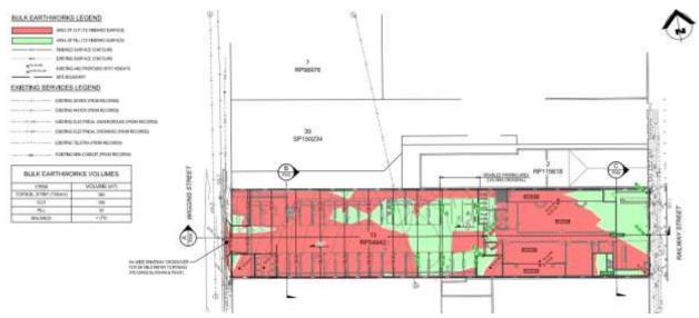
Figure 3: Preliminary Earthworks Plan
