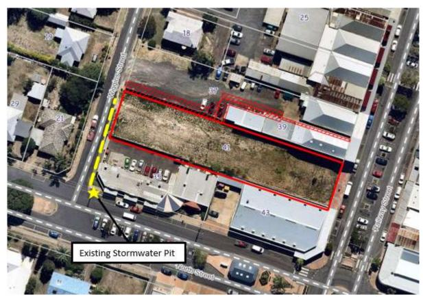
Figure 4: Existing stormwater pit and underground stormwater system (yellow dashed line) to be provided
