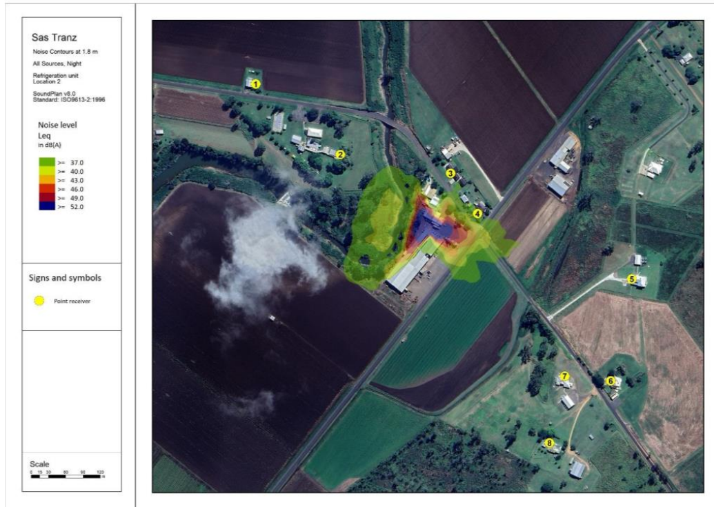
Noise contours at 1.8m, night-time cumulative variable noise sources. Levels are in dB(A), L_{eq}
