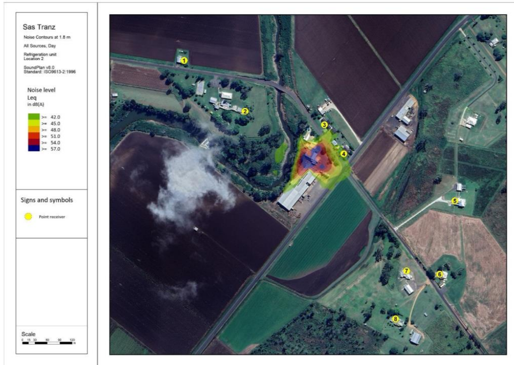
Noise contours at 1.8m, daytime cumulative variable noise sources. Levels are in dB(A), L_{eq}
