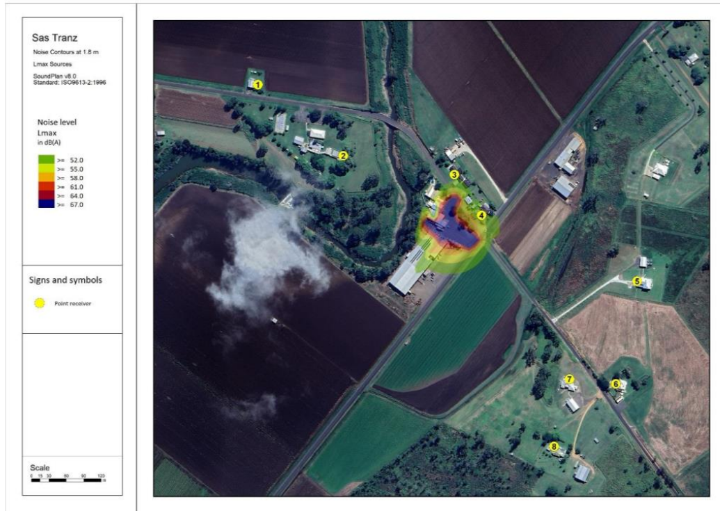
Noise contours at 1.8m, night-time cumulative discrete noise sources. Levels are in dB(A), L_{max}
