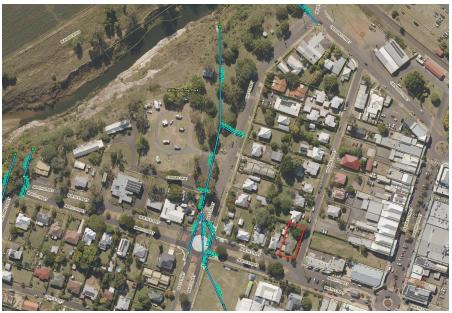
Figure 3 – Existing Stormwater Infrastructure
