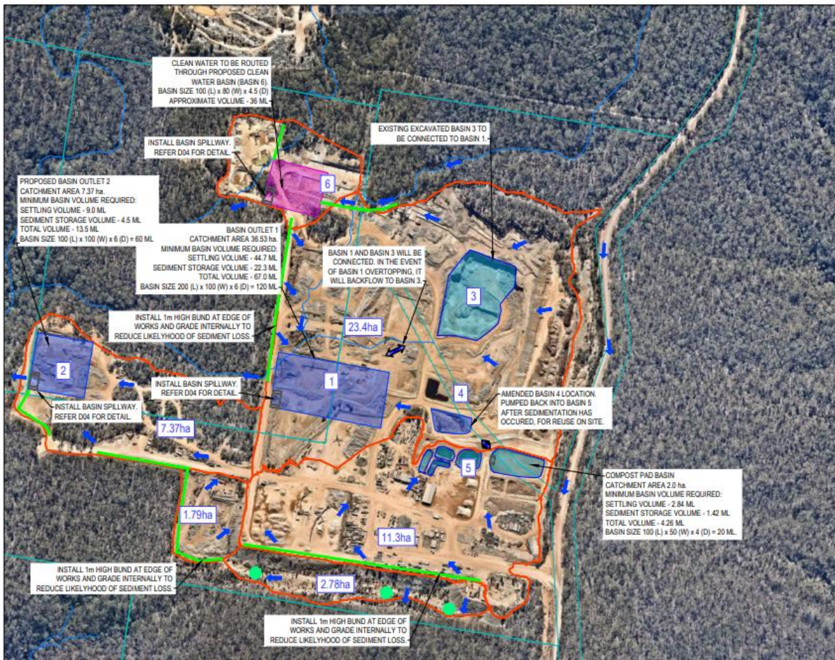
Figure 10. Extract of Stormwater Management Plan showing Drainage Plan
